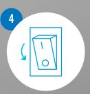
Flip the On/Off switch to Off. Take off protective equipment.
